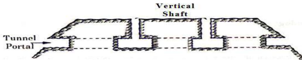
Fig. 1.1 : Tunnel Driving With Help of Vertical Shafts
